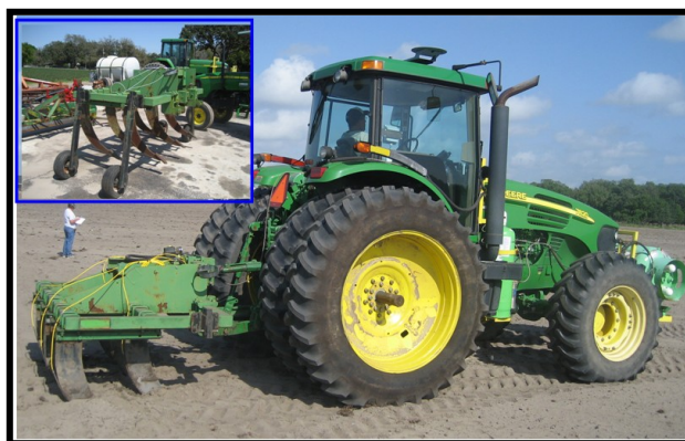
Figure 2. Subsoiler being used to destroy highly compacted, subsurface traffic pan and to deliver fumigants 20-24 inches deep into soil. Authors would like to acknowledge gratefully that the subsoiler was provided courtesy of Jimmy Moden, Hendrix & Dail, Palmetto, FL.
