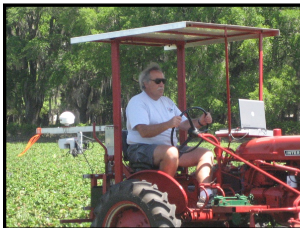
Figure 1. New tractor (1964) and remote sensing equipment being used to characterize and map sting nematode distribution and damage by row within strawberry fields.
