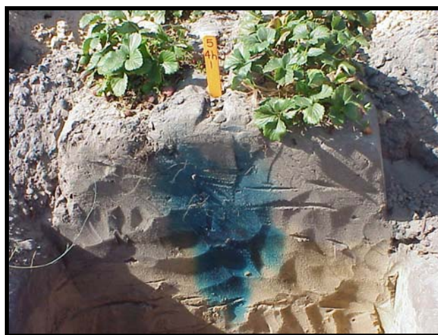
Figure 1. Cross-sectional view of a strawberry bed using a blue dye to map movement of irrigation water in soil from a single drip tape after a four hour injection period.
