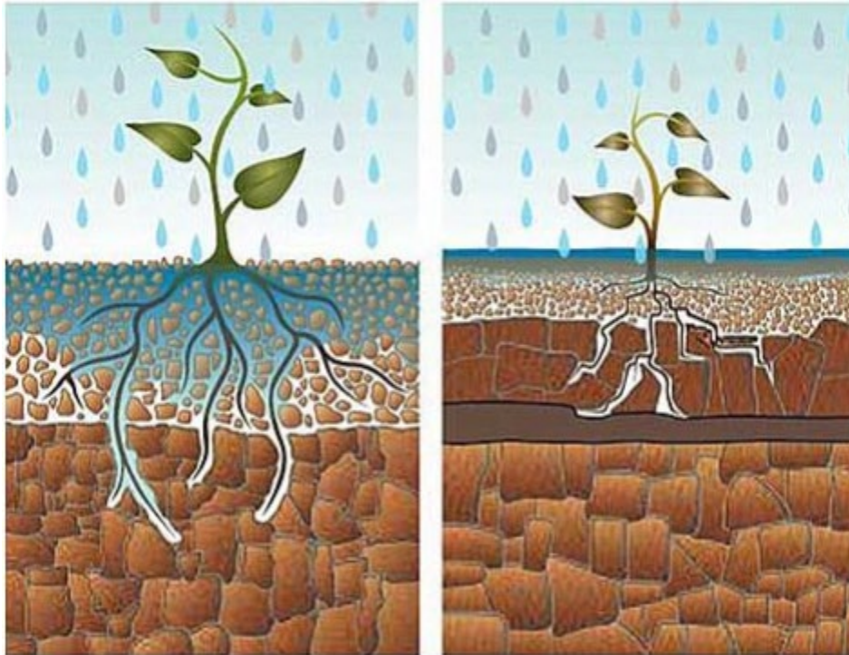
Figure 1: Illustration of a good Soil (Left) and a Compacted Soil (Right) (Image credit: Forigo roteritalia, 2019)
